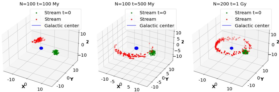
FIGURE 6. Formation of a tidal stream. Time advances from left to right as indicated. A blob of order 100 point stars (green) at  $t = 0$  is stretched by the tidal field of a sphere+cylinder gravitational source with the parameters of our Milky Way galaxy. Because of a small initial  $v_z$  vertical velocity, the simulated stream is seen to acquire a torsion.
