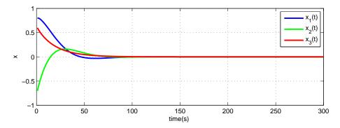
Figure 3.1: Evolution of the states  $x_1(t)$ ,  $x_2(t)$  and  $x_3(t)$  with the initial conditions  $x_1(0) = 0.8$ ,  $x_2(0) = -0.7$ ,  $x_3(0) = 0.6$ , and  $\alpha = 0.98$ .
