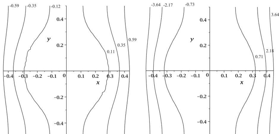
**Fig. 2** Temperature distribution in the cell  $Q_{(0,0)}$  for the nonlinear composite, with the average flux intensities  $|A| = 30$  and  $|A| = 100$ .
