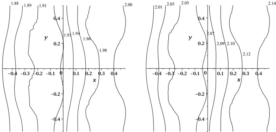
FIG. 12. Temperature distribution inside the cell  $Q_{(0,0)}$  calculated during utilisation of the second method described in the Subsection 5.2. The results correspond to the constants  $C = 27$  and  $C = 28$ , respectively.
