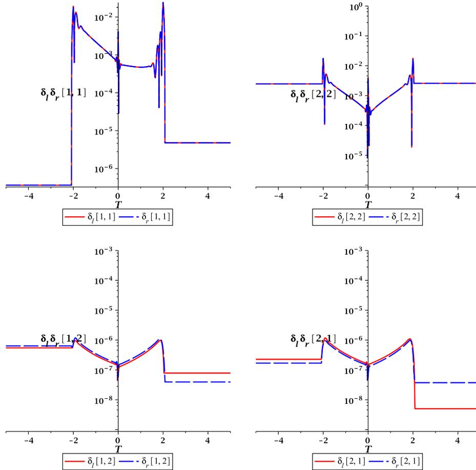
FIG. 11. Relative difference between components of the tensors  $\delta_l$  and  $\delta_r$  from (6.2) showing the perfect matching between the formulae for effective properties of the periodic and random composites.
